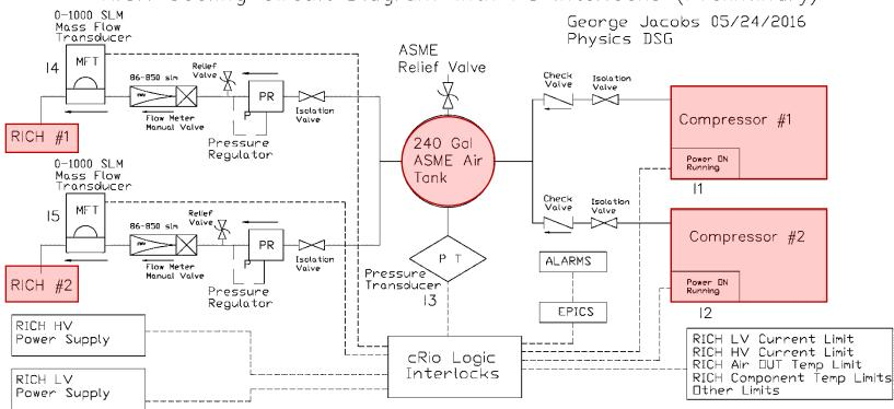
Cooling Circuit Interlocks for RICH HV and LV Power to be Enabled Air Compressor Power ON Interlock - 11 and/or 12 or PS Power is Disabled Air Pressure Interlock - 13 > 100 psi (TBD) or Power Disabled Air Flow Interlock RICH #1 Power - 14 > 250 slm (TBD) or Power to RICH #1 Disabled Air Flow Interlock RICH #2 Power - 15 > 250 slm (TBD) or Power to RICH #2 Disabled
