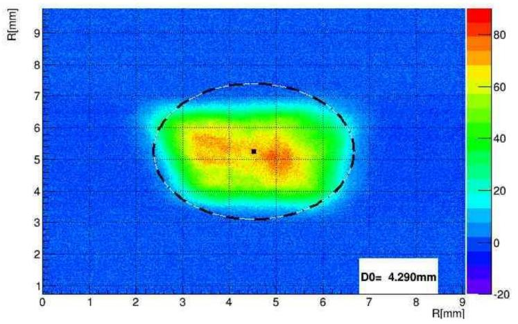
Spot distortion because spot is not at focal plane
